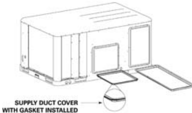
Figure 22. Duct cover with gasket installed
